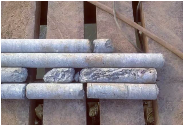
图7 基桩钻芯法混凝土取样 Fig.7 Concrete sampling by pile core drilling method
