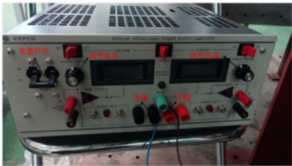
图8 EECD 的外部电源连接装置 Fig.8 External power connection device of EECD
