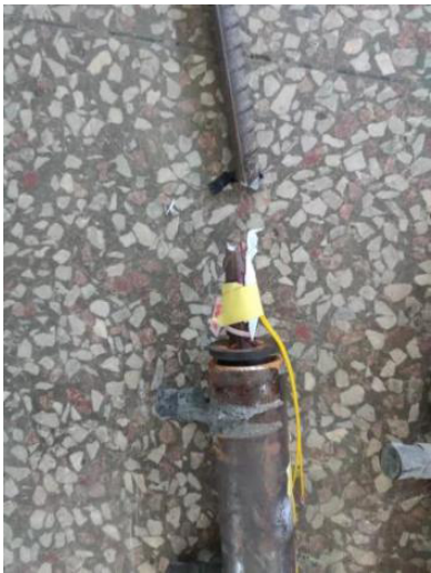
(a)钢筋拉断破坏
