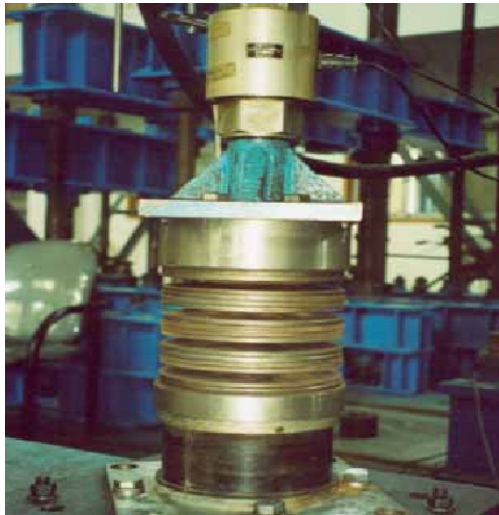
图 10 三维隔震支座力学性能试验 [49] Fig.10 Mechanical performance test of 3D seismic isolation bearing [49]
