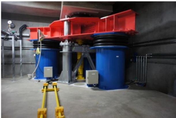
图 12 空气弹簧与支座组合的隔震装置 [58] Fig.12 Shock isolation device combined with air spring and support [58]
