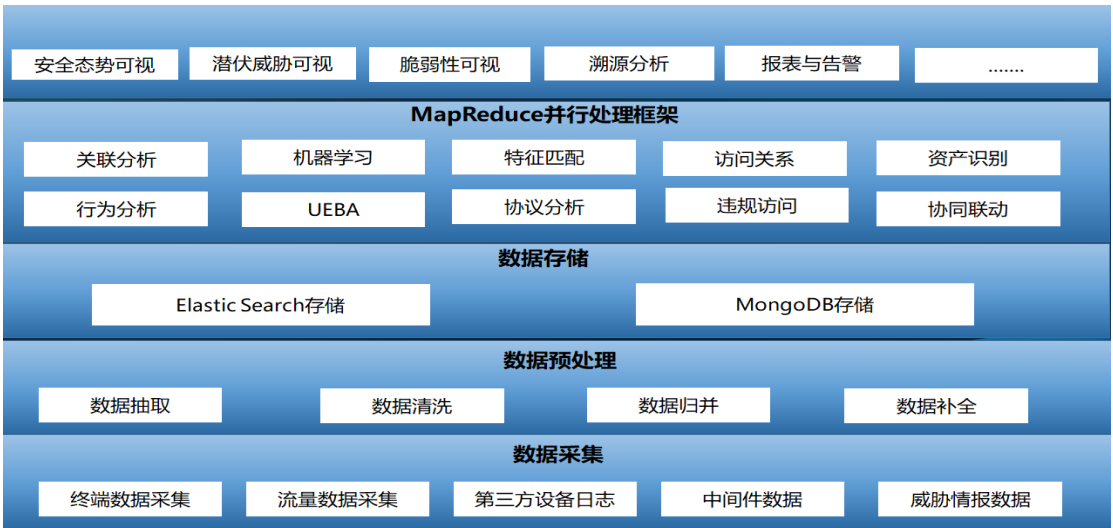
图2 安全感知平台架构图 Fig.2 The architecture diagram of safety awareness platform
