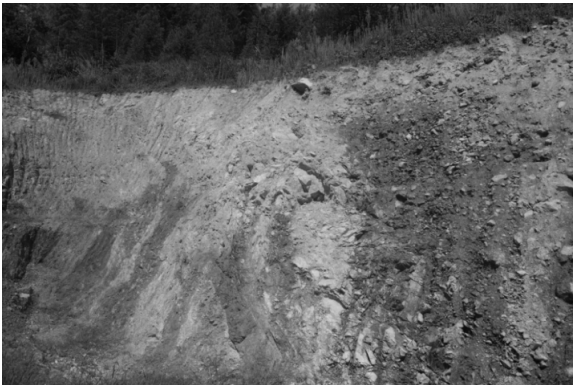
①坡积物；②凝灰岩；③ 断层破碎带夹断层泥
