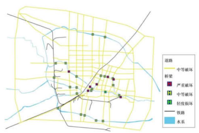
图3 IX度地震烈度下桥梁震害预测结果 Fig.3 Seismic damage prediction results of bridge under IX intensity
