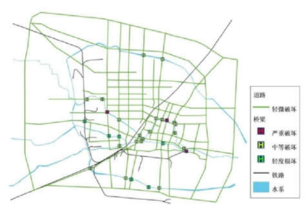
图2 VIII度地震烈度下桥梁震害预测结果 Fig2 Seismic damage prediction results of bridge under VIII intensity
