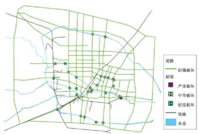
图1 VII度地震烈度下桥梁震害预测结果 Fig.1 Seismic damage prediction results of bridge under VII intensity
