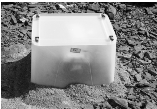
图 8 测点仪器第一层防护罩图 Fig.8 The picture of the first protective cover for the observation instruments
