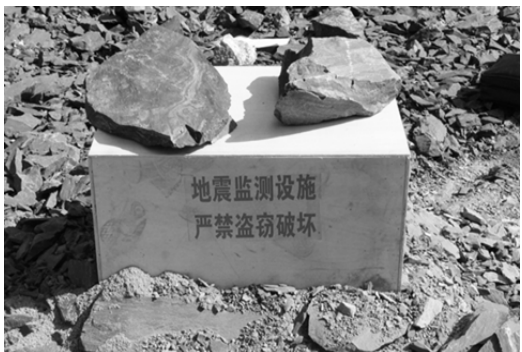
图 9 测点仪器第二层防护罩和警示标语图 Fig.9 The picture of the second protective cover and warning signs for the observation instruments
