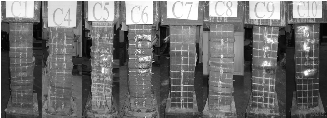
图 5 各试件的破坏形态 Fig.5 Collapse forms of the specimens
